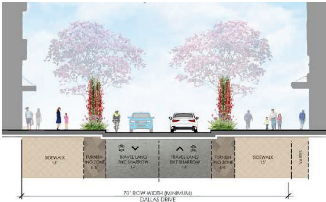
Figure 2-11: Dallas Drive Cross Section
